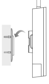
4. Hook the router onto the bracket and slide it downwards until it locks into place.
