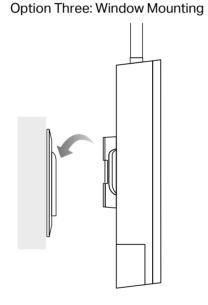
2. Hook the router onto the bracket and slide it downwards until it locks
