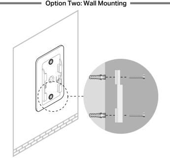
3. Tap the two wall anchors into the holes. Align the bracket with the wall anchors and install the two self-tapping screws to secure the bracket. Ensure the mounting bracket is not installed in the wrong direction.
