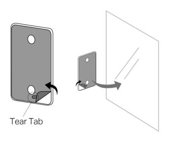
1. Tear off the release paper of double-sided adhesive tape and stick the bracket on the window. Apply slight pressure to ensure stronger bond.
