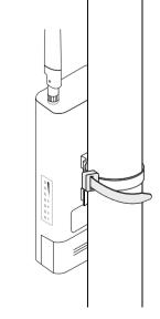
2. Position the router and wrap the pole mounting strap around the pole. Feed the end through the screw-block and tighten the strap until the router is secure.
